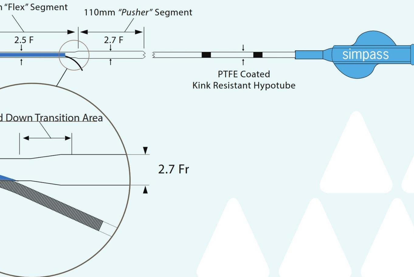
Conical Shaped Shaft Tip For CTO Lesions
